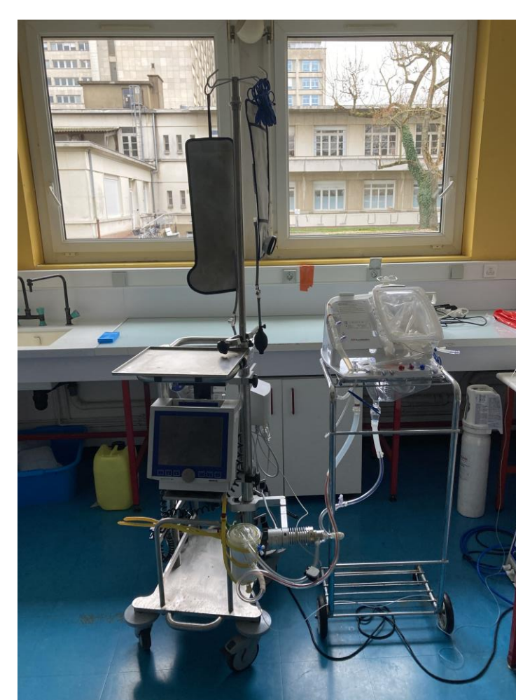
Figure 2 (left) et 3 (right). Homemade NEVHP set-up. Left - Homemade ex vivo heart perfusion circuit composed of a repurposed OCS™ console (right) and a pulsatile MEDOS ECMO pump/oxygenator (left). Right - OCS™ console with porcine heart
